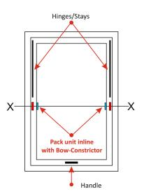
Bow-Constrictor must be fitted centrally at the points X-X to achieve the best seal
